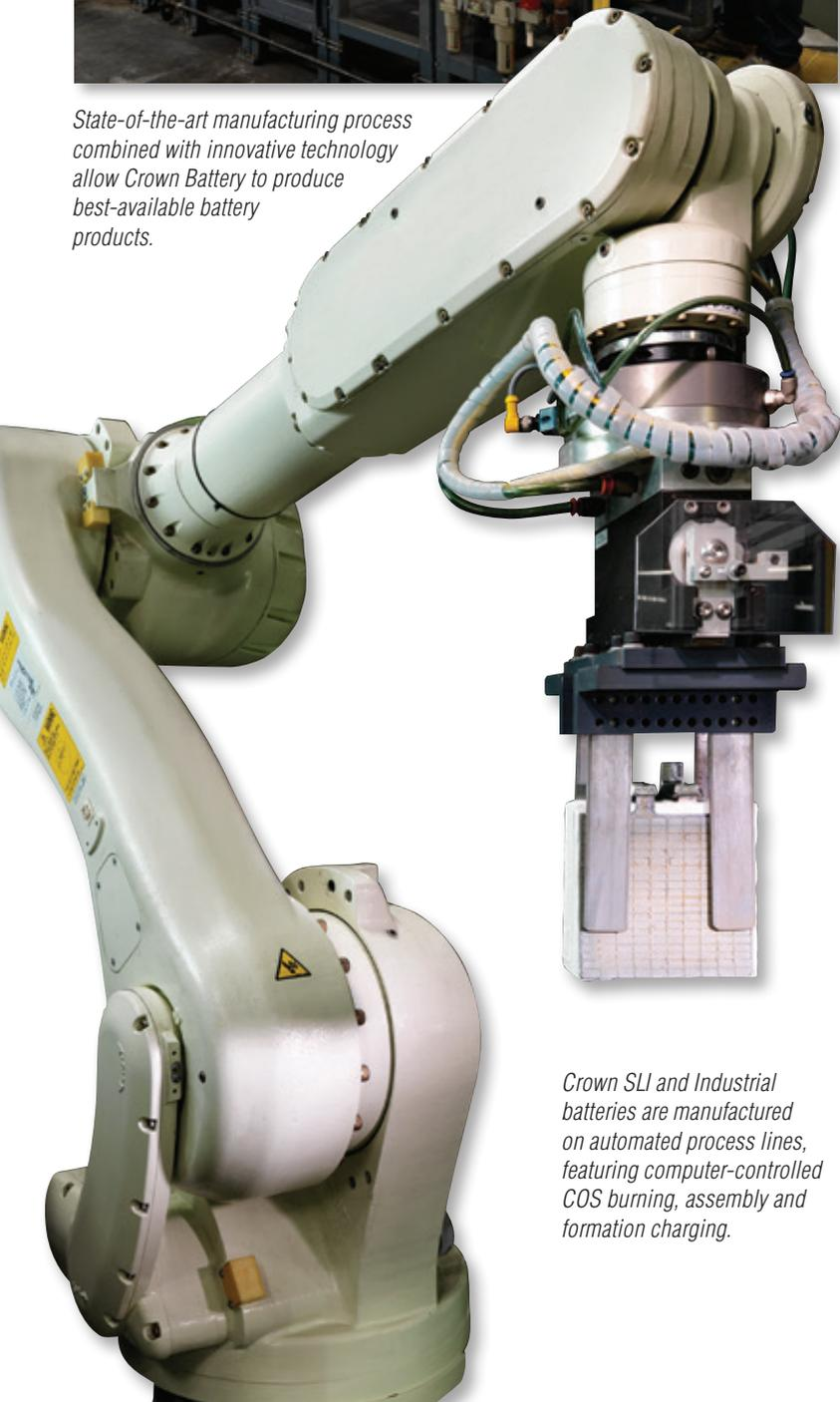
*Crown SLI and Industrial batteries are manufactured on automated process lines, featuring computer-controlled COS burning, assembly and formation charging.*
